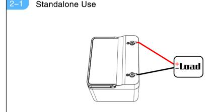
Connect one end of the positive and negative wire harness to the positive and negative poles of the battery respectively. Use the matching M8\*12 triple combination screw to fix it, and then connect the other end of the wire harness to the positive or negative pole of the load respectively (do not reverse the connection, which may cause safety hazards or damage to the battery and equipment).
