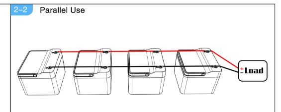
This product supports up to 4 batteries in parallel. Before using the product in parallel, the batteries to be connected in parallel must be fully charged (the charger turns green), and the screws matching the product must be connected according to the figure above for parallel use (positive pole to positive pole; negative pole to negative pole) and insulation of the terminal at the connection must be done.
